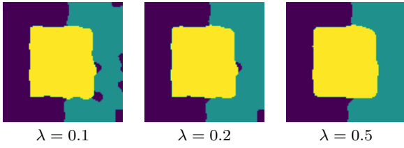
Fig. 7: Results for different values of the regularization parameter \lambda corresponding to the segmentation problem depicted in Figure 6. Holes in the segmentation mask disappear by enlarging the regularization parameter.
