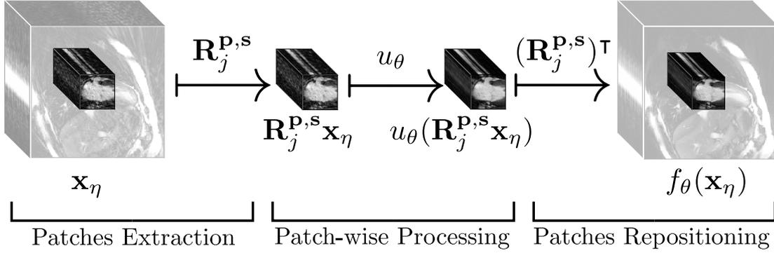
Figure 1: Workflow for obtaining a CNN-prior by patch-based processing: First, the initial reconstruction is divided into patches, then the network  $u_\theta$  is applied to all patches. Reassembling all processed patches results in the CNN-prior which is then used for regularization of the inverse problem.
